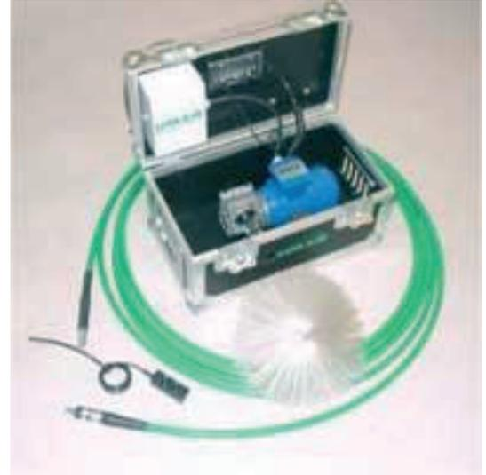
The Lifa Special Cleaner 2 is an electric wire brushing machine.
