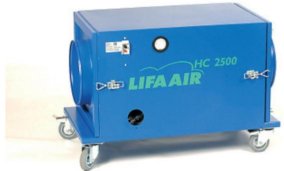
HepaClean 2500 is intended for cleaning dry air containing asbestos, mould, construction, quartz, powder or wood dust. When the machine is equipped with an active carbon filter, gaseous compounds can be removed. The machine can also be used to create negative pressure in rooms and compartments.
