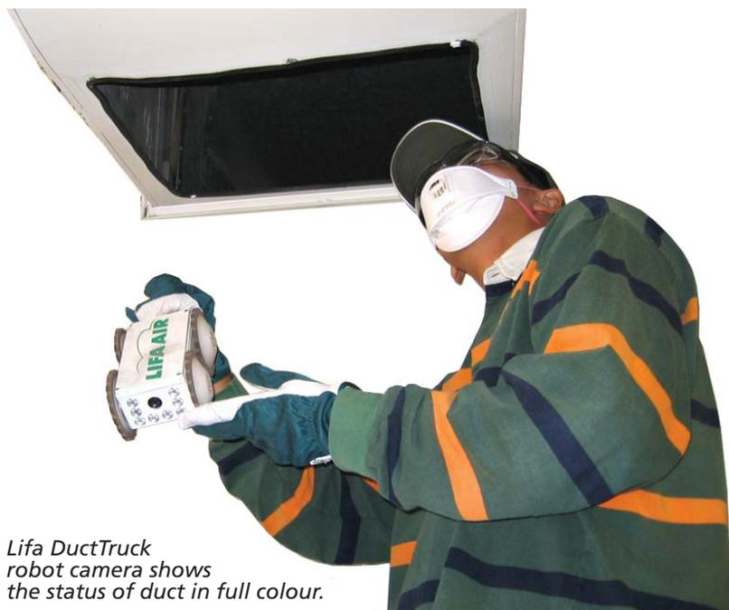
Lifa DuctTruck robot camera shows the status of duct in full colour.
