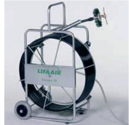
The Lifa AirJet Combi 20 is a compressed air blowing machine designed mainly for disinfection and for spraying coating substances on the inside surface of ventilation ducts. It can also be used for loosening and removing the kind of dirt that does not adhere strongly to duct surfaces. The Lifa AirJet Combi 20 blowing machine is a cleaning machine ideally suited to areas that cannot be reached with a brushing machine. The 20-meter (66 ft.) long axle guarantees extensive reach.
